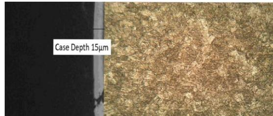
Fig 5: Vacuum tempering specimen (600°C)
