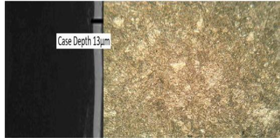
Fig 4: Vacuum tempering specimen (500°C)
