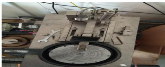
**Fig 2:** Pin on disc apparatus
