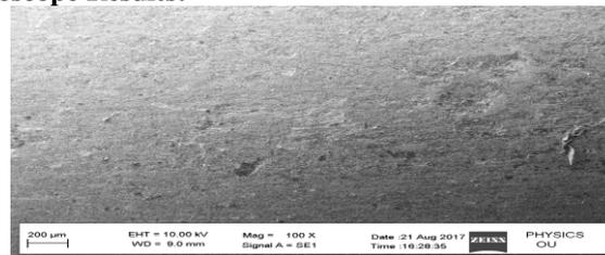
Fig 6: Vacuum tempering specimen (500°C) at 100X
